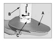
Reassemble the filter parts (as shown in the figure) and reinsert the whole assembly into the dishwasher. Position it into its housing and press downwards. The dishwasher is not to be used without filters. Improper replacement of the filters may reduce the efficiency of the wash and even damage your dishwasher.
